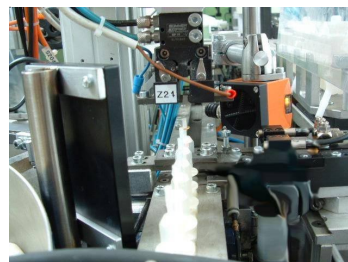
Mounting of a washer of the fuel tank float, being checked using the principle of colour separation
