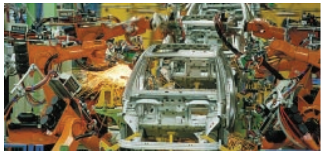
Pneumatics application in the unpainted body shell area when the welding tongs need to be transported, held, gripped and fed.
